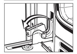
Flip down the locking clamps on each door hinge. This locks the hinges.
